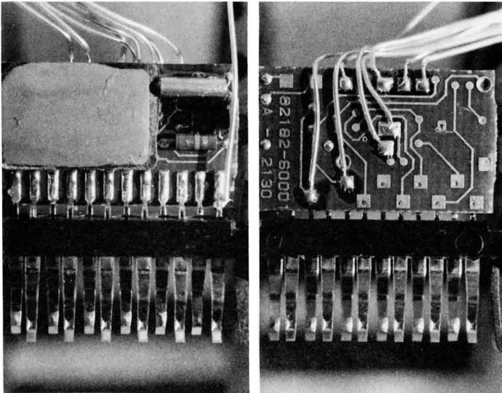
**Figure 3-1:** Photos of Phineas, the nickname for the time module, when cracked open. The left photo (3-1a) shows the front view; the rear view on the right (3-1b) reveals previously unknown solder pads which can be used for interacting with the outside world.
