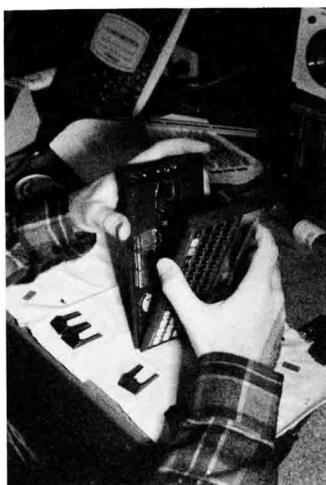
**Open the 71 this way**, with the ON key pointing up. The old version has a fragile ribbon cable at the bottom, which should be treated as a hinge.
