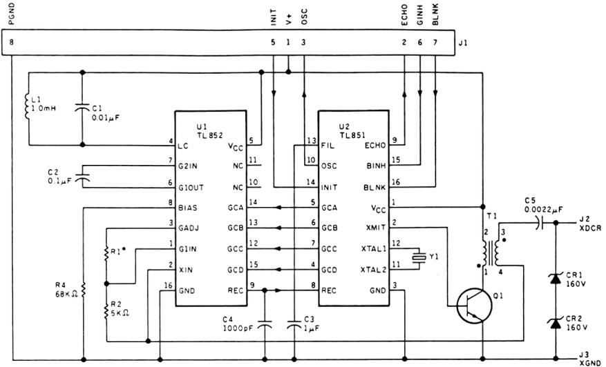
A schematic of the circuit is shown in Fig. 9-1 above. What makes this module so wonderful is that it will automatically increase its sensitivity to the returning echo the longer it waits; extending its measurement range. Even better is it only takes four wires to interface the unit to a computer. (And two of them are power!)
