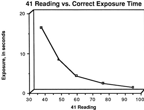
This table is used to determine the proper exposure given a reading of an 18% grey area of the desired negative. The equation describing this graph turns out to be:
