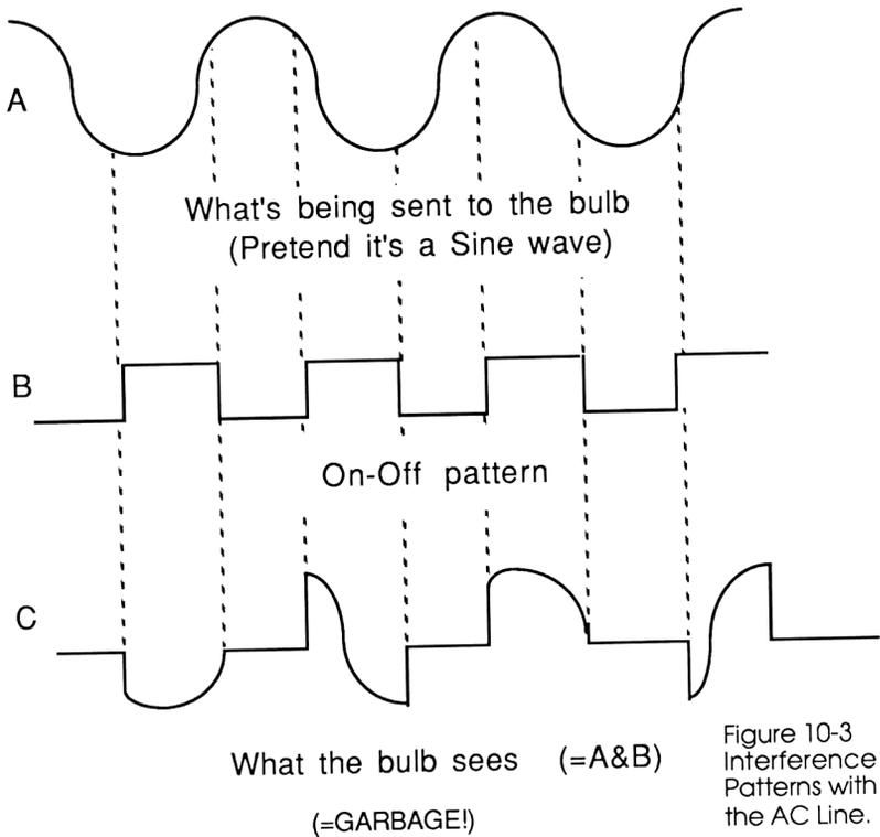
the AC lines, and make the bulb's output look like there's an intermittent break in the AC cord, rather than the constant illumination we're so used to seeing.
