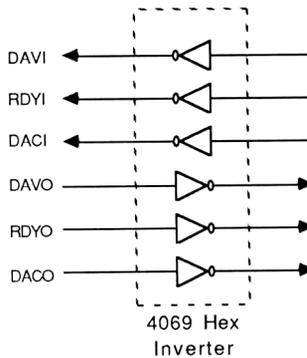
A Simpler Way Which Works on All 8-Bit Ports.
