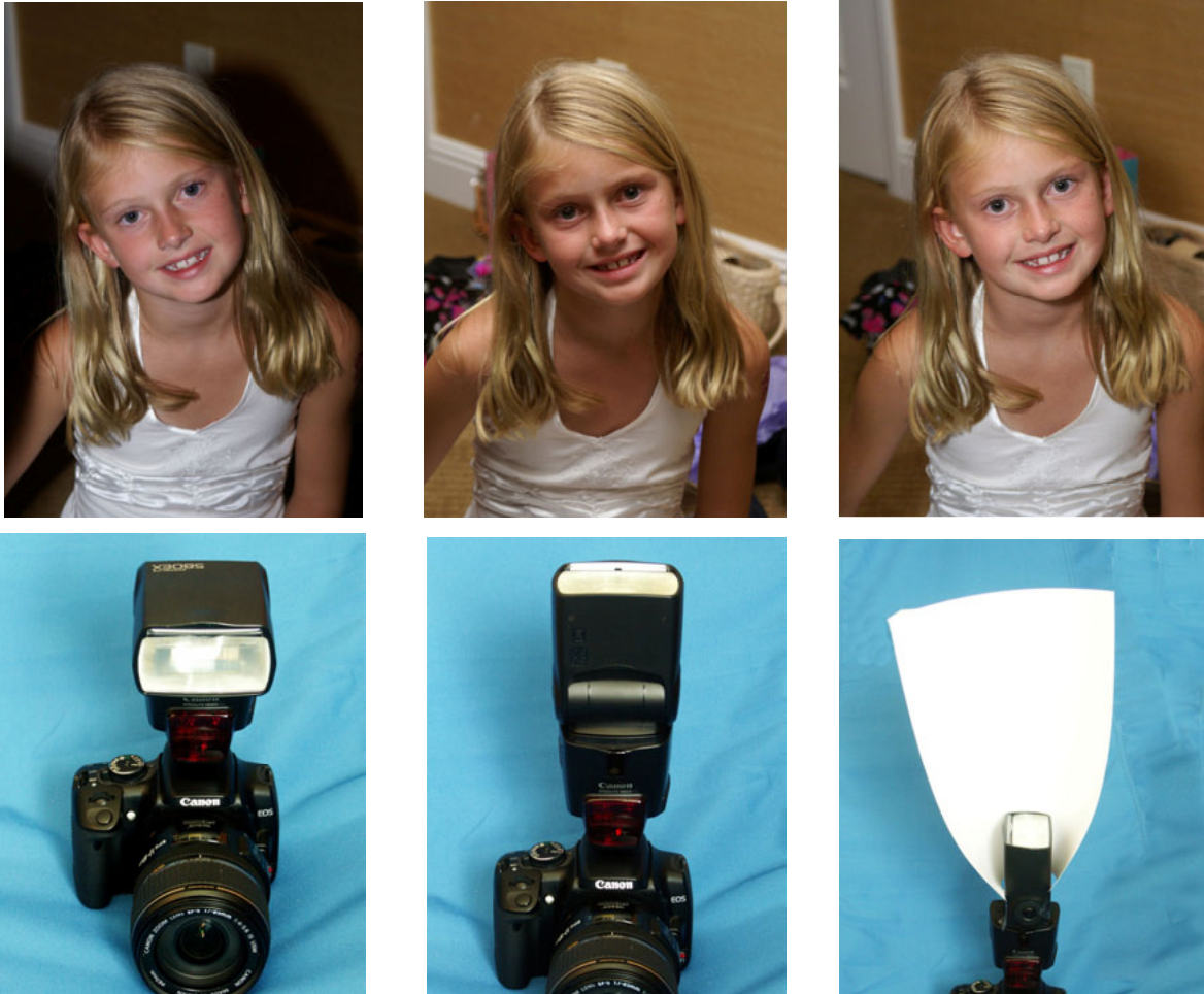
Figure 7-18: Examples of Straight on-camera flash (Yuk!) vs. ceiling bounce. The third picture uses an easy-to-make light modifier which takes some of the light destined for the ceiling and converts it into a soft, pleasing subject light. What a difference!
