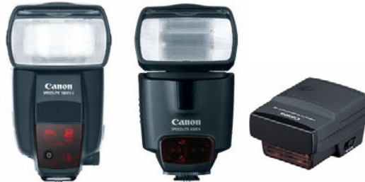
Figure 7-2: To use wireless mode, you'll need two EX-series flashes (such as the 580EX or 430EX (left and center), or at least one EX flash and the ST-E2 infrared transmitter (right). One device sits on the camera's hot shoe, and the other may be positioned almost anywhere around the room. Not all EX flashes can act as a "Master", however. See the next section for more information.
